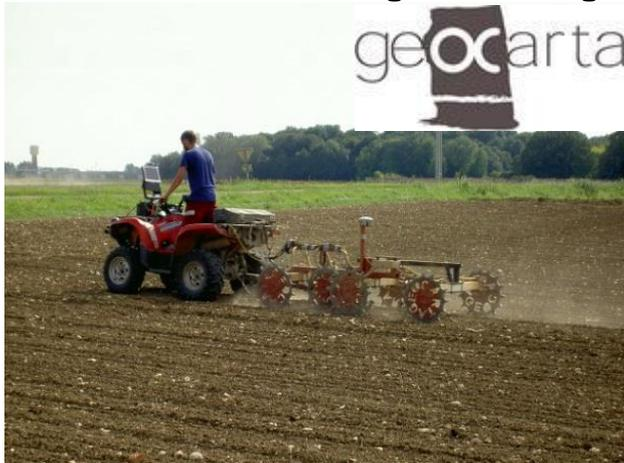
**L'ARP (Automatic Resistivity Profiler) :**
